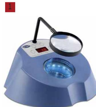
**Scope of supply:** Device with two Wolffhuegel graticules and dish centering adapters to facilitate use with 50 to 90 mm dishes.
